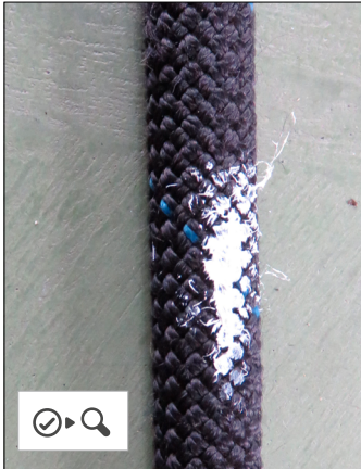
• Trace of paint
