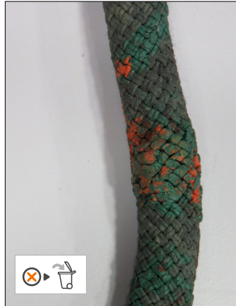
• Trace of paint
