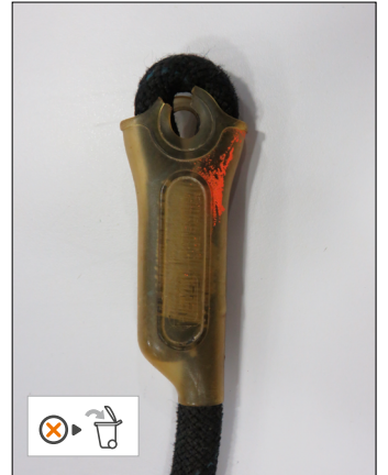
• Damaged plastic sleeve
