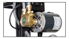
Your SG2 system comes with a direct drive rotary vane pump. This pump has graphite vanes which push the water through your system. **Do not run the pump dry.** Running the pump without water could result in damage to these vanes and a loss of pump function.
