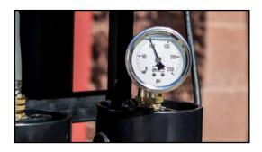
The SG2 comes with an inline pressure gauge. You can move the inline to any of the garden hose connections on the system to take readings. We recommend you attach the pressure gauge to the inlet of the DI filter cartridge. Do not run system with the DI filter pressure above 100 PSI.
