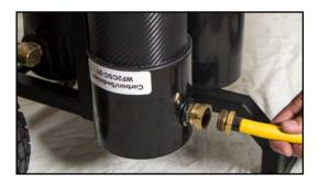
Your SG2 is designed to be operated while standing up. Locate an external water source. Attach one end of the feed hose (not supplied) to the water source. Open the faucet at the building and make sure all air is out of your source hose. Turn off water and attach to the female connection on the Carbon/Sediment filter. Turn water back on fully and adjust bypass valve to desired flow rate.
